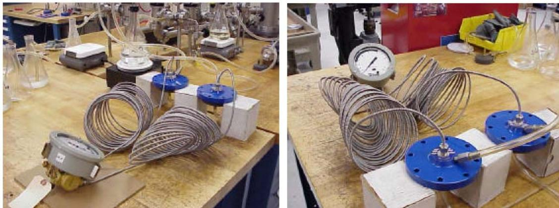
As in the direct mount version, the maximum vacuum will be reached at some point, normally within one hour. At this point the fill tubes will be lowered into the selected fill fluid, the system vented to the atmosphere, and the fill fluid is drawn into the evacuated instrument. Once the unit is completely filled, the secondary vacuum is released, and the bleed ball and screw are installed.
