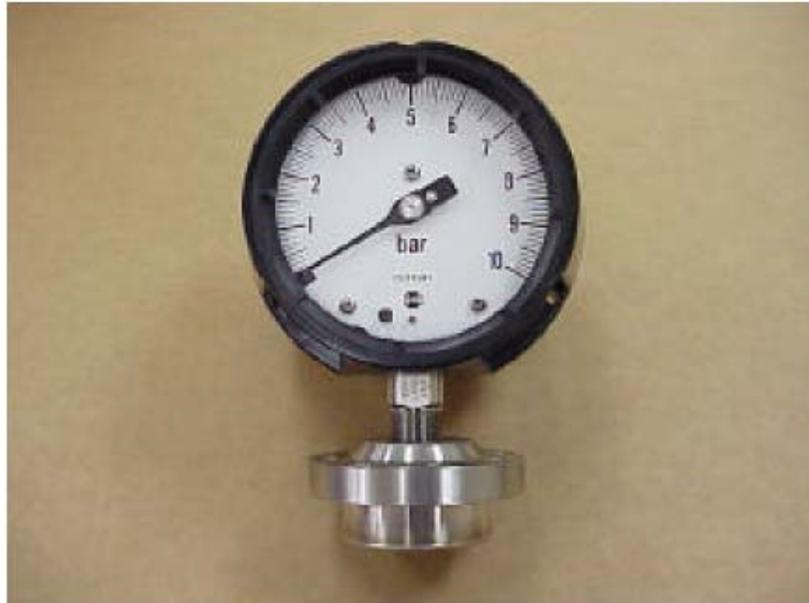
You now have completed an instrument directly mounted to a diaphragm seal fill application.
