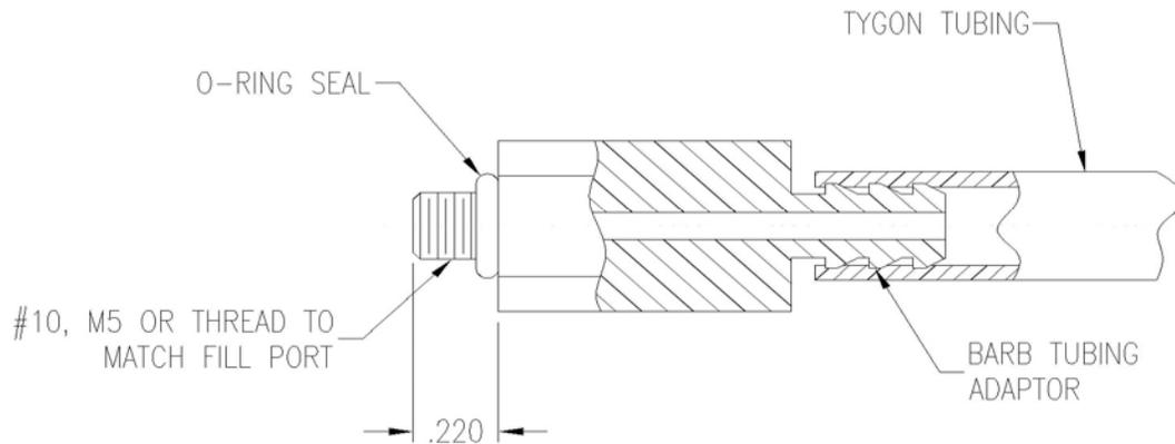
Using a quality vacuum pump, attach the diaphragm seal instrument assembly by using ¼” tygon tubing. Initiate vacuum pumping of the diaphragm seal and instrument assembly. Evacuation times will vary due to the size of assembly and the fill fluid selected. Plan on evacuating for 20 minutes. Periodically check assembly to make sure there are no vacuum leaks.
