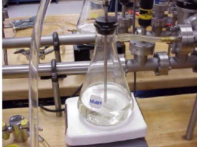
Closing off or isolating the vacuum source from the instrument assembly will allow you to open your control valve, enabling the fill fluid to be drawn into the evacuated area. Back filling time of the instrument assembly will vary depending on the viscosity of the fill fluid being used. Usually this time will be less than 50% of the evacuation time.
