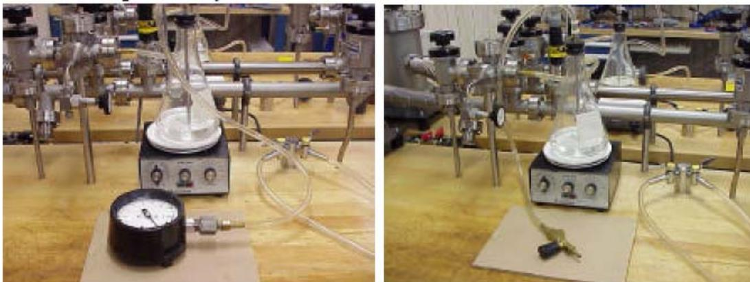
The diaphragm seal, however, is filled in a completely different manner. Inspect the diaphragm seal to be filled, remove the bleed screw and bleed ball.
