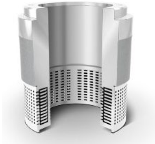
Figure 6 Globe Valve Cage Trim Utilizing Pressure Staging for Aerodynamic Noise Attenuation
